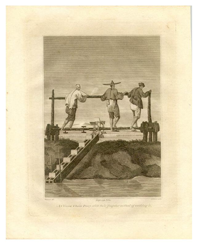
*Figure 2*. A dragon's backbone tool for irrigation, commonly used in China. It is also known as a square-pallet chain pump. Pumps like these helped farmers reap more rice, but they also increased the labor requirements.
